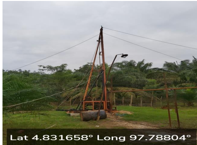
Sumur Tradisional Metode Air Lift
