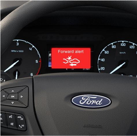
Autonomous Emergency Braking (AEB) with Pedestrian Detection<sup>1</sup>
