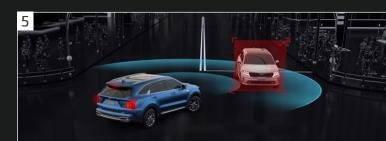
**5-** Designed to monitor and detect vehicles or vulnerable road users travelling ahead of you, the Autonomous Emergency Braking system automatically applies the brakes if it determines a crash<sup>7</sup> is imminent, helping to avoid a frontal collision. The Junction Assist function will help avoid a collision with an oncoming vehicle in an adjacent lane when turning right at an intersection.
