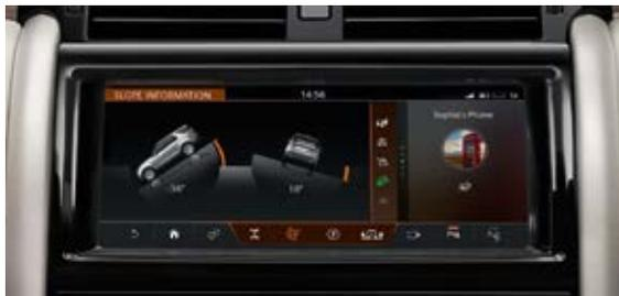
The All Terrain Info Centre within your navigation system allows you to view and activate various features and provides access to All Wheel Drive (AWD) information and guidance features for off-road driving.
