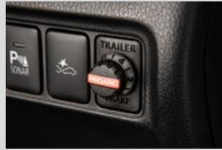
Electric Trailer Brake Controller with Harness
