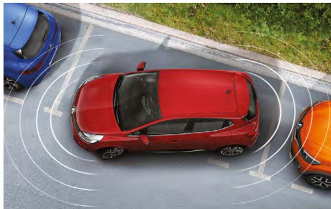
The hands-free parking system has 12 sensors placed on the front, rear and sides to detect a spot with adequate dimensions to park your vehicle.
