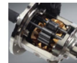
On muddy or snowy surfaces, one wheel may slip or be lifted into the air. In this case, the locking differential forces both wheels on an axle to turn in unison, allowing the vehicle to recover its traction.
