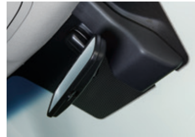
Front camera module (AEB/LDW/LKS/HBA/TSR)with rain sensing and automatic
