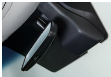
Front camera module (AEB/LDW/LKS/HBA/TSR) with rain sensing and automatic light control unit
