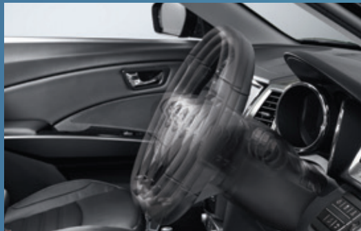
Telescopic and tilting adjustable steering wheel
