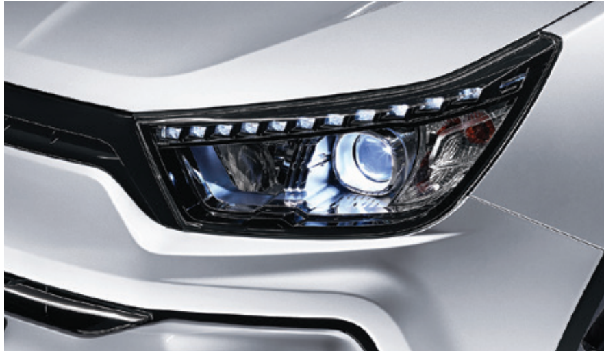
HID head lamp assembly crowned by a series of LED daytime running lights
