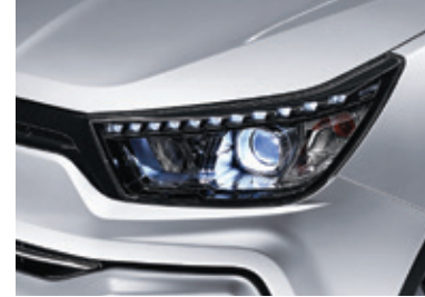
HID headlamp with LED day time running lamps
