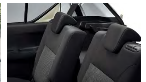
EASY SLIDING REAR SEATS The left and right rear seats slide forward and backward separately from each other, making it possible to adjust for legroom, luggage and all sorts of situations (LTD).
