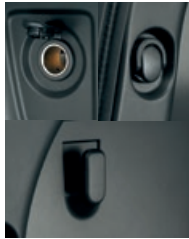
Extra convenience: The luggage area incorporates a 12V DC power socket and hooks for holding luggage in place.
