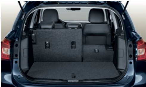
Flexible space: Even with five people aboard, there's 430 litres of luggage space. By folding down the 60:40-split rear seatback, you can expand the space in diverse ways. A multi-position luggage board gives even greater flexibility.
