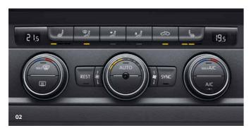
**O2 Optional "Climatronic" air conditioning system.** This system offers 2/3-zone temperature control for the driver, front passenger and living area. The automatic air recirculation function, air quality sensor and optional auxiliary heater all work together to create a pleasant interior climate.
