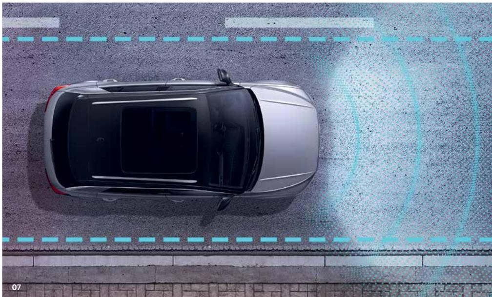
**06** The **Blind spot sensor** can alert you to vehicles in your blind spot (within the system's limits) so that you don't change lanes. When you're reversing out of a parking space, the **Rear Traffic Alert** monitors the areas behind and to the side of your vehicle and warns you if there is traffic crossing your path.
