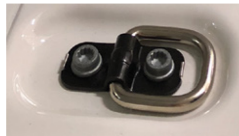
The lashing eyes are recessed to lie flush with the floor.
