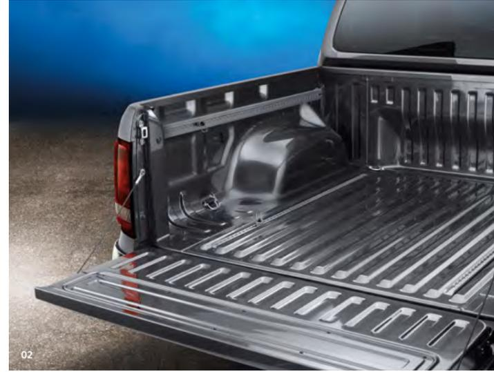
**01 The widest load platform.** No other diesel ute provides so much space between the wheel housings: the loading width of 1,222 mm even enables standard pallets to be loaded crosswise. The spacious cargo box with a 2.52 m<sup>2</sup> load surface features convincing dimensions – such as the 508 mm high side panels and the low loading sill height of 780 mm. **S**
