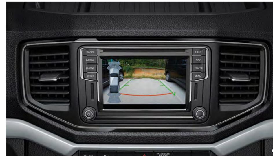
**04 "Rear View" reversing camera** simplifies parking by showing a limited view of the area behind the vehicle on the display. Static guidelines facilitate the parking process. **S**
