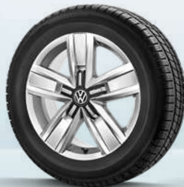
17-inch "Devonport" alloy wheel. 1) 7 J x 17. With 235/55 R 17 tyre. | BE | CO | OC |
