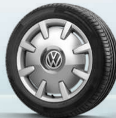
18-inch "Disc" alloy wheel. 2) 8 J x 18. Silver surface. With 255/45 R 18 tyres. | BE | CO | OC |
