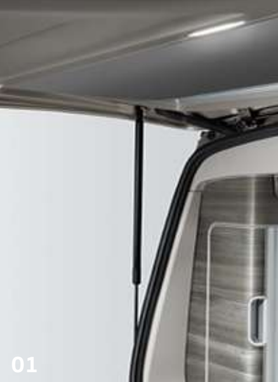
01 Tailgate spotlights. Two LED lamps on the inside of the tailgate provide more light in the living compartment when it is dark outside. When the tailgate is open, the luggage area and the area behind the tailgate is illuminated to facilitate loading and unloading. | BE | CO | OC |
