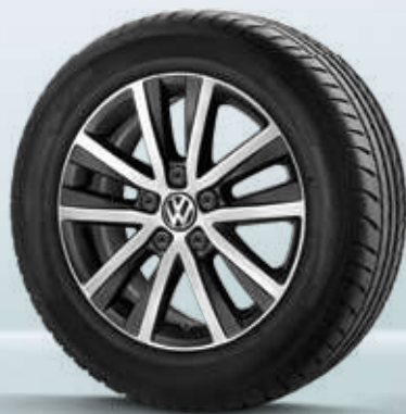
17-inch "Cascavel" alloy wheel. 7 J x 17. Burnished surface in black. With 235/55 R 17 tyre. | BE | CO | OC |
