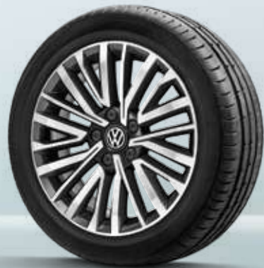
18-inch "Palmerston" alloy wheel. 8 J x 18. With 255/45 R 18 tyre. | BE | CO | OC |
