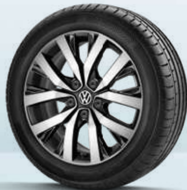
18-inch "Toluca" alloy wheel. 8 J x 18. With 255/45 R 18 tyre. | OC |
