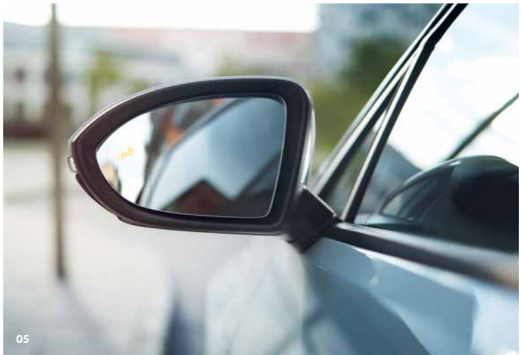
05 Blind spot monitoring using sensors, this genius feature informs you when a vehicle is in your blind spot, with illuminated symbols on each of your side mirrors.
