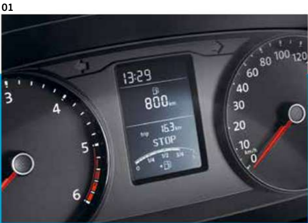
01 Start/stop system. After shifting into neutral and releasing the clutch*, the engine is switched off automatically, e.g. at red traffic lights. To start the engine again, it is enough to step on the clutch.
