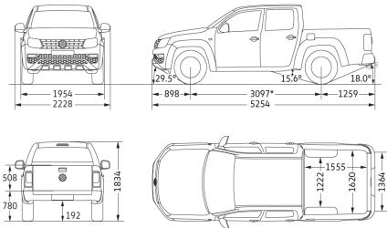
$\mbox{{\sc *}}\mbox{This}$  value applies for unladen weight. When loaded, the wheelbase is 3,090 mm.
