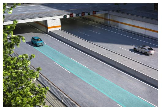
01 Lane Assist uses a camera to monitor the markings on the road ahead, and helps keep you safe by working to prevent you leaving your lane unintentionally. It employs small steering corrections to keep the vehicle in the correct lane. Works from a speed of 60km/h within system limits.
