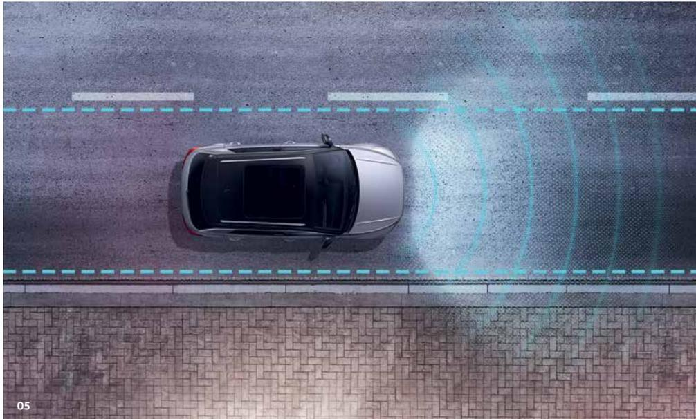
**04** The **Front Assist** monitoring system combines Pedestrian Monitoring with City Emergency Braking, alerting you if it detects vehicles or pedestrians at the edge of the road, via acoustic and optical signals, as well as a gentle application of the brakes. The system even performs an emergency stop should the distance become critical, helping to protect other road users and possibly avert potential accidents.<sup>2)</sup>
