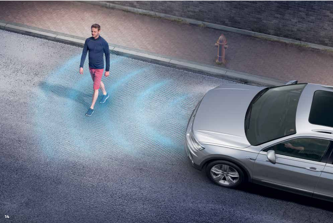
13 The Area View Camera supports the driver when exiting concealed exits or side streets, when entering or driving out of parking spaces. It generates a 360 degree surround view on the touchscreen and provides a bird's eye view.
