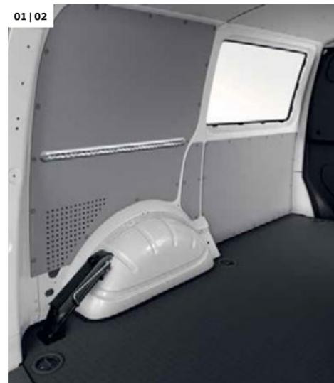
**01 High side panel trim (hardboard).**<sup>1)</sup> Full-height protection of the side panels from the floor to the roof frame. | KA | KO | KP |
