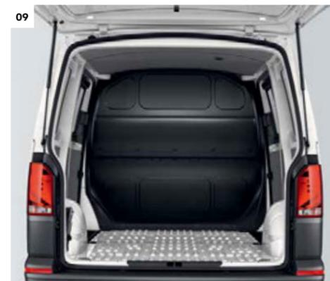
**09 High partition, closed.** Fully separates the load compartment from the cab. | KA | KO |
