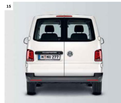
**15 Rear wing doors with window.** Extend the field of vision thanks to a narrow centre pillar in combination with extra-wide windows. Standard for the Kombi with high roof. | KA | KO | KP |
