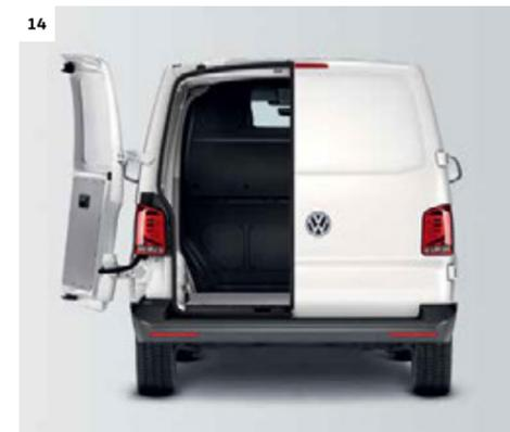
**14 Rear wing doors.** Rear wing doors are standard for models with high roof. | KA | KP |
