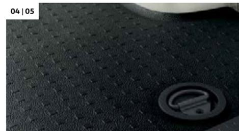
**04 Anti-slip, washable rubber floor.** Increases safety through an anti-slip surface that extends over the loading sill and the step lighting. | KA | KO | KP |
