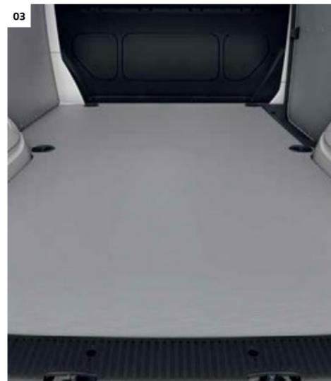
**03 Universal floor (for fittings).** The ideal preparation for subsequent installation of cabinet systems from various manufacturers.<sup>3)</sup> Special adapters<sup>4)</sup> in the recesses in the floor covering permit flexible installation of cabinet systems at any time without gluing or drilling. Subsequent removal of the floor leaves only minimum traces. | KA |
