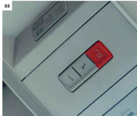
**03 eCall.** After an accident, automatically transmits the time, position and number of vehicle occupants to the emergency call centre and establishes a voice connection. The system is activated by a crash sensor or manually via the emergency call button. Available with the Composition Colour radio system and above. | KA | KO | KP | PR |
