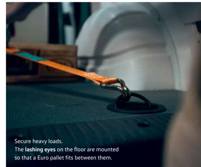
Secure heavy loads. The lashing eyes on the floor are mounted so that a Euro pallet fits between them.
