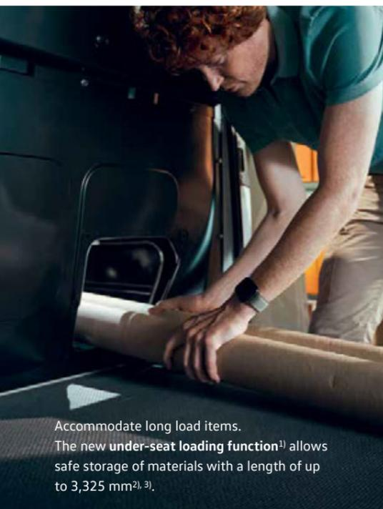
Accommodate long load items. The new under-seat loading function<sup>1)</sup> allows safe storage of materials with a length of up to 3,325 mm<sup>2)</sup>.<sup>3)</sup>
