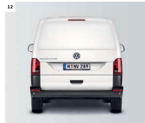
**12 Tailgate without window.** Allows convenient loading and unloading with a large opening height of max. 2,200 mm<sup>8)</sup>. | KA | KP |
