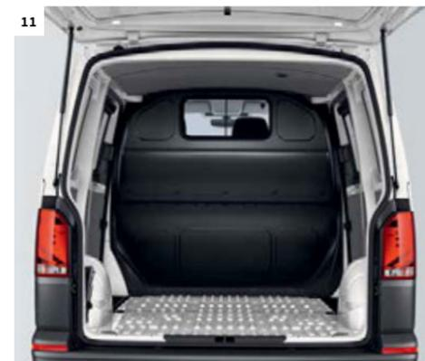
**11 Partition, high with sliding window.** Offers a flexible opening between the cab and load compartment. | KA | KO |
