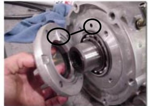
Once you have verified that you have the same style input gear, install the gear into the planetary, install the snap ring. Re-install the planetary assembly into the case and secure the input to the bearing with the front snap ring. **Note:** The only part you should have left out of the case is the old input gear. During reassembly, make sure the oil return hole matches the front retainer hole.
