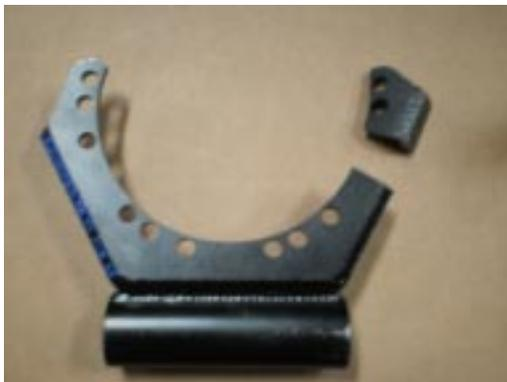
The mount needs to be cut to provide clearance for the transfercase shifter linkage bracket.
