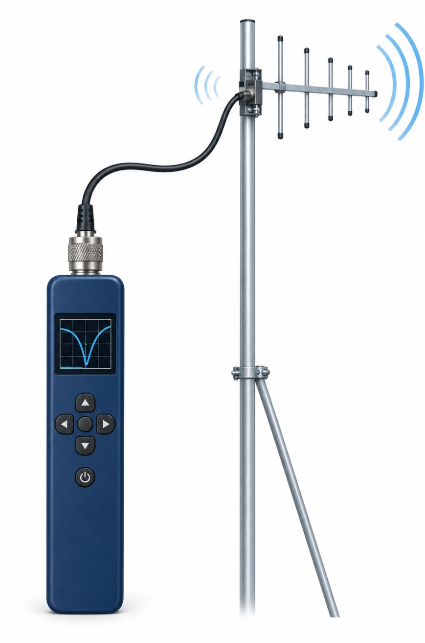
Figure 1. The analyzer sends a small test signal down the coax and uses the returning signal to describe the antenna and cable.
