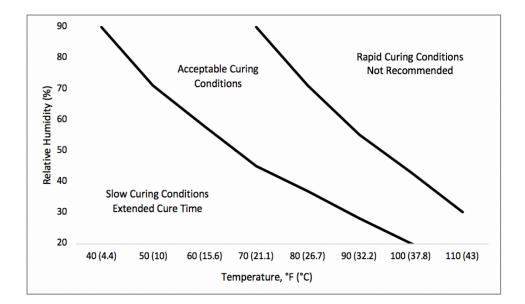
Chemglaze A074 may be recoated after the first application within 4 hours minimum and 24 hours maximum when cured at room temperature [25°C (77°F)] and 50% relative humidity. The recoat time is dependent on temperature and humidity. High temperatures and humidities promote fast cure while low temperature and humidity slow down the cure. For maximum intercoat adhesion, recoat within 24 hours.
