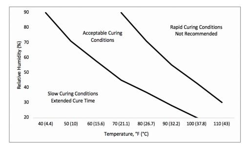
Chemglaze A080 may be recoated after the first application within 4 hours minimum and 24 hours maximum when cured at room temperature [25°C (77°F)] and 50% relative humidity. The recoat time is dependent on temperature and humidity. High temperatures and humidities promote fast cure while low temperatures and humidity slow down the cure. For maximum intercoat adhesion, recoat within 24 hours.
