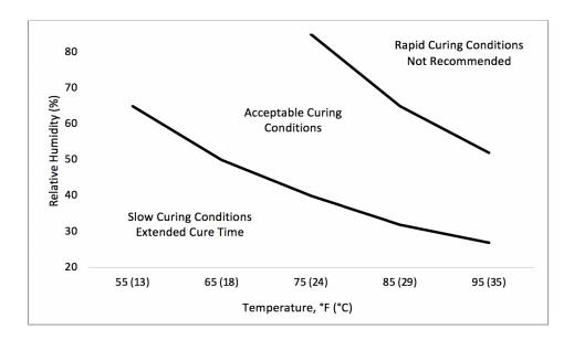
Chemglaze V209 cures to a tack-free surface in 2-18 hours at room temperature depending on the application thickness, catalyst, and relative humidity. Faster handling times can be achieved by using one of the following cure cycles:
