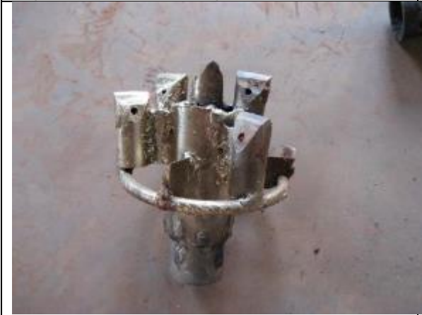
A new drill bit for the SHIPO drill system with Tungsten bits.
