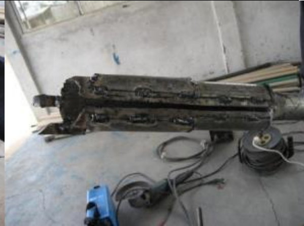
The Soil punch was reinforced to reduced breakage
