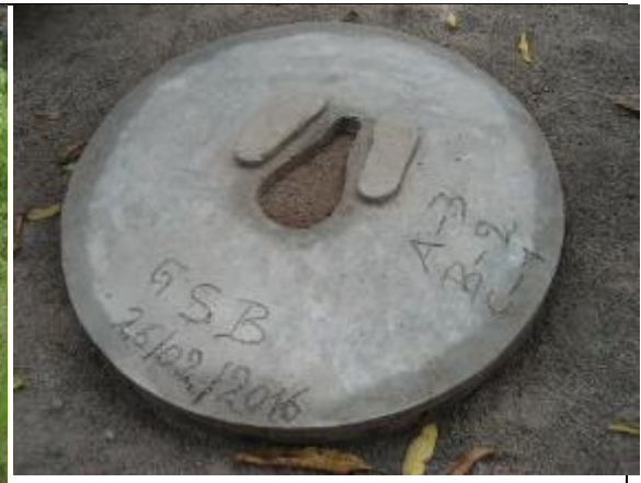
In the Santolic program GSB trains village masons in making latrine slabs.
