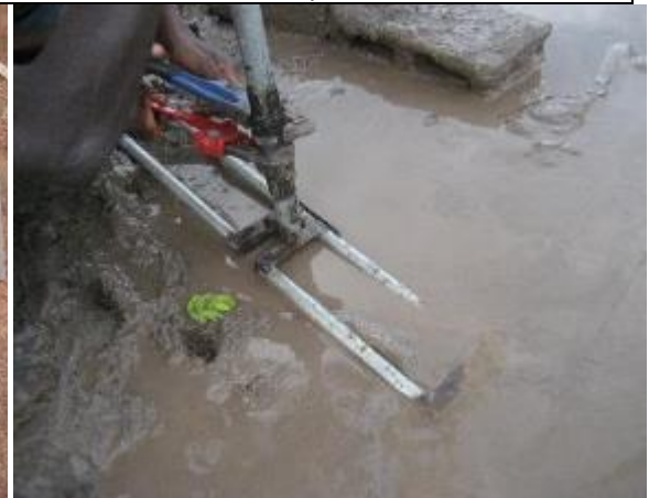
The Grip has 2 pipes instead of a bolt and fixed with a rubber strip
