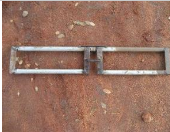
Support for drill pipes to keep the pipes hanging while changing the drill pipe
