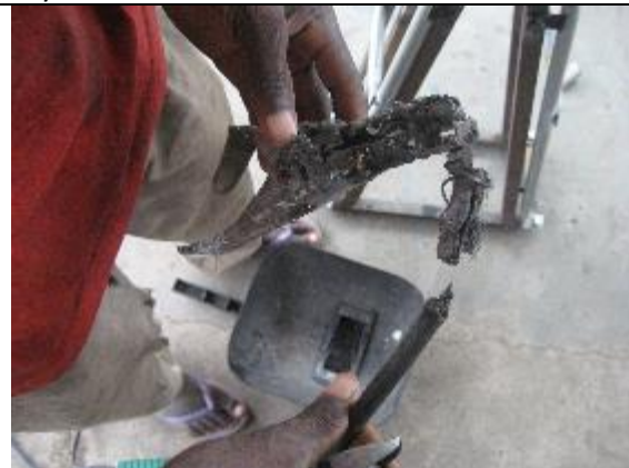
One of the problems is quality in the workshop. Here worn out and broken welding cable
