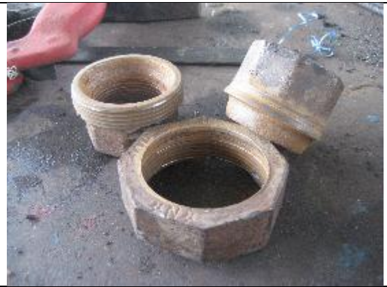
Swivel. This type of Swivel was worn out in 2 days so other solutions are needed
