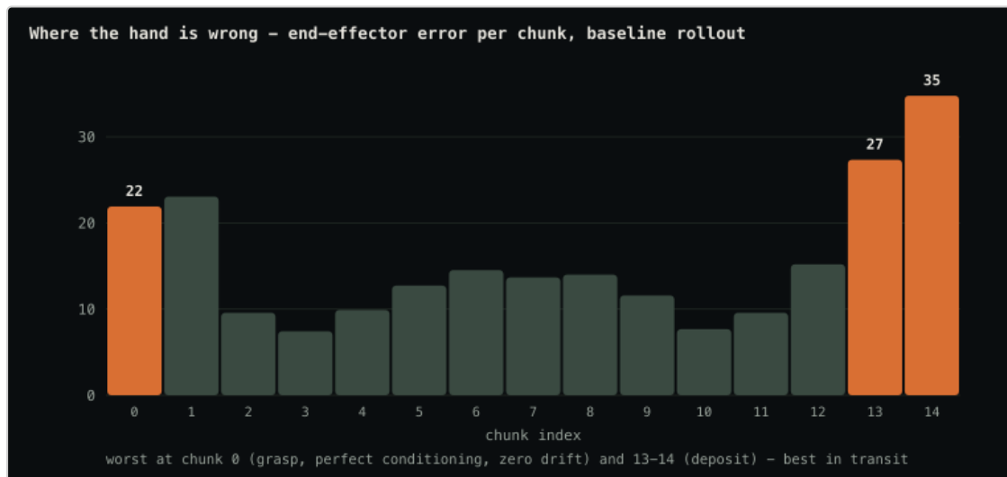
Figure 1 — end-effector error per chunk on the baseline rollout, held-out ep52. Chunk 0 has a real photograph as conditioning and zero accumulated drift, and is still among the worst chunks in the episode.
