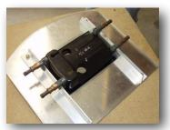
Using at least two Cleco® edge clamps, clip the Panel Dock to the rails. This will allow you to determine how it should look from the front before you drill any holes.
