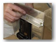
The bolts we provide have an integral washer on the screw-head side. This provides adequate distribution of force on the plastic to keep it from cracking.
