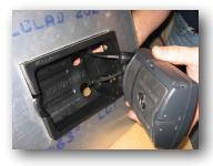
The Panel Dock has been designed to allow the cables that are included with the GPS to be used. There are "keyholes" in the back of the Panel Dock to allow the cables to be inserted with the unique feature of keeping the cables from disappearing behind the panel when the GPS is removed. If desired, you may cover the larger holes using rubber grommets.
