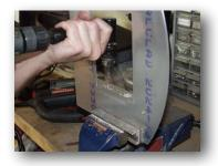
There are a number of ways in which you may choose to drill the holes. You can remove the rails from the panel and drill them on a drill press, or you may use an angle drill to drill them in the plane. Just be careful to make accurate holes at the marks you made, and you will be fine. Use a 3/16 inch drill bit to drill the four mounting holes.
