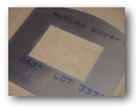
The panel cut out dimensions for the the Panel Dock should be 6.25 inches wide and 4.25 inches tall. See the cut template on the Panel Dock specification sheet and measure your Panel Dock to be certain. On the provided template, note that paper can expand or contract with the weather.
