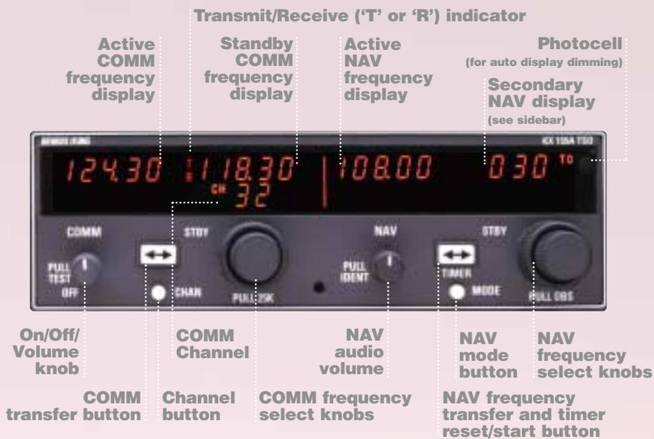
from-station mode. An internal Course Deviation Indicator (CDI) has been included for those times when an external CDI is being driven by your GPS receiver, and the systems now include a handy elapsed-time and approach timer. The KX 165A features a built-in VOR/LOC converter, enabling it to directly drive a horizontal situation indicator (HSI).
