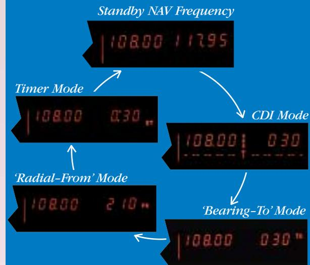
*The KX 155A & KX 165A incorporate five different NAV operating modes which can be changed by simply pressing the NAV Mode button.*
