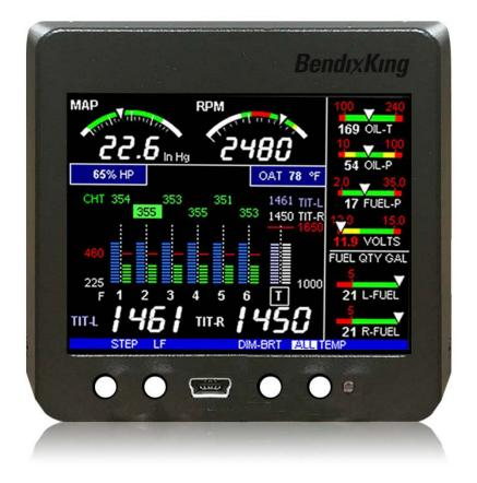
The xPoint 100 is a high-resolution / low-cost piston-engine indication system for experimental aircraft. Extremely compact, with a starting cost of \$795, this advanced solution provides incredible resolution and legibility packaged in a 13-ounce unit.
