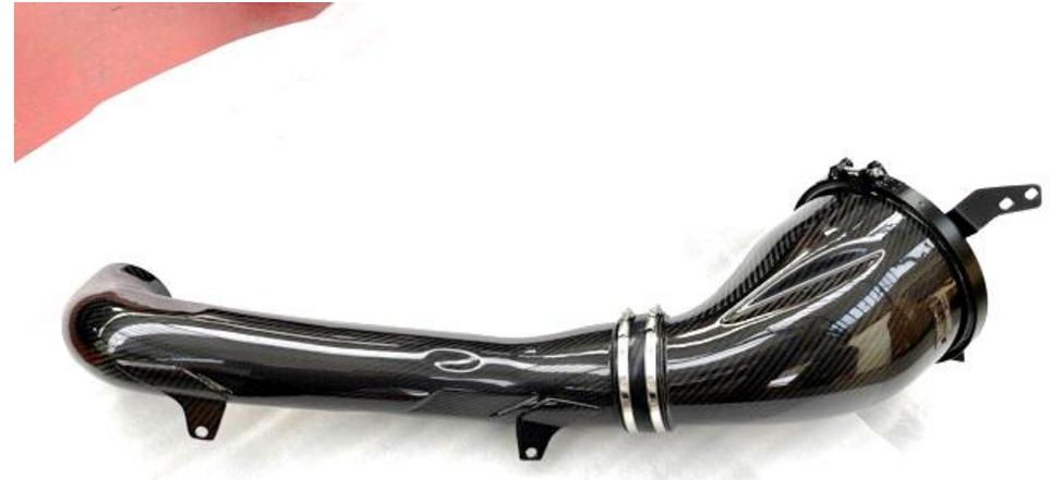
33. Assemble the carbon tube and RHS housing as shown using the supplied silicon hose and 2 x 100-120 clamps . The RHS housing has a bracket attached to the front and curves
