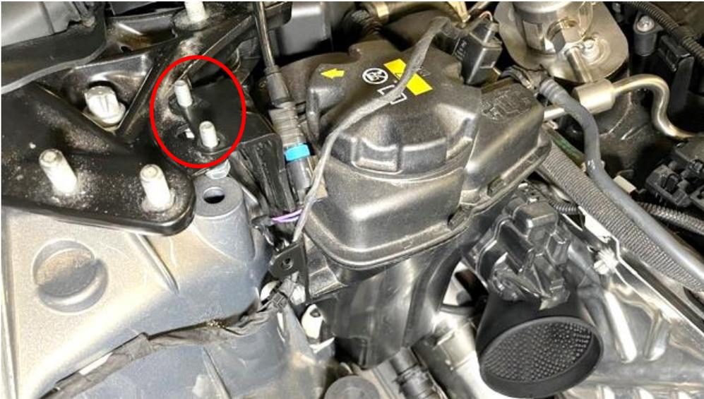
52. For more clearance we now need to move the coolant tank. Remove the 2 x 10mm nuts on the coolant bracket shown.
