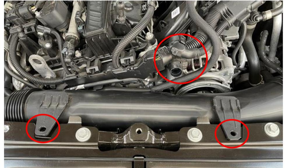
6. Unclip the plug shown to allow more clearance for the tube. Also remove the 2 plastic push clips in the tube brackets.
