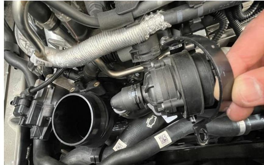
10. For better access, remove the bracket shown around this module. Bracket is held in place by a 10mm nut. You can then move the module away from the inlet for better access to the screws.
