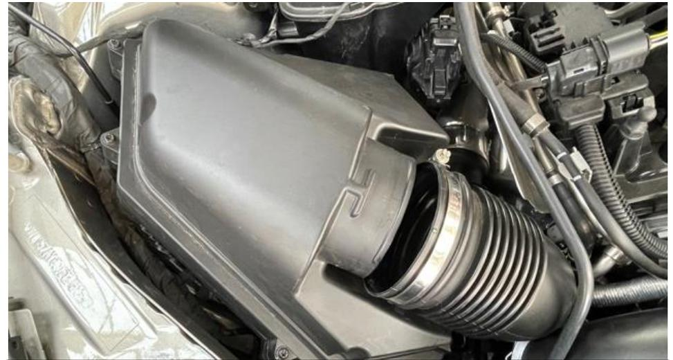
2. Starting with the left side (as you look at the engine from the front of the car) loosen and remove the flexible tube from the airbox. The Pull the airbox out - it is held in with rubber grommets.
