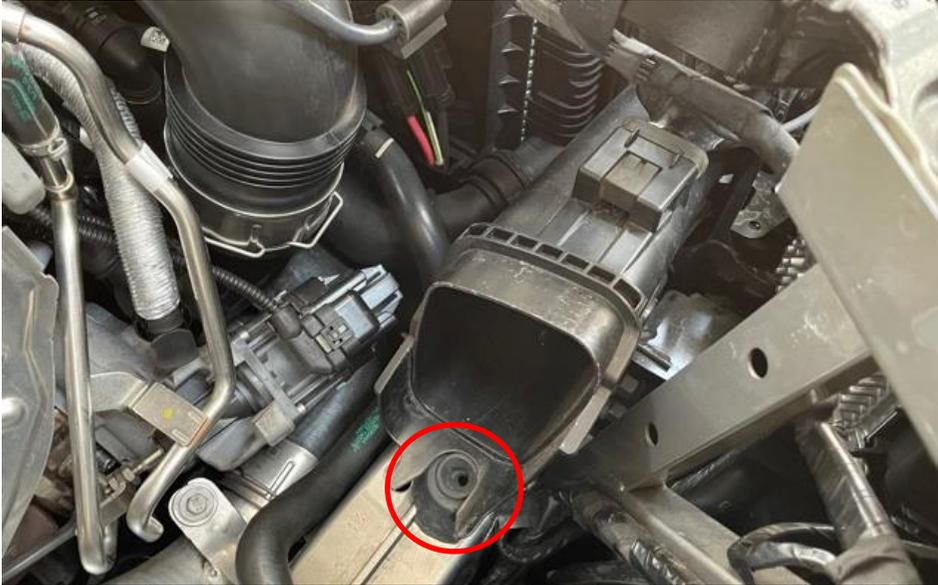
5. Remove the air duct and also the rubber grommet circled. The air duct simply pulls out.
