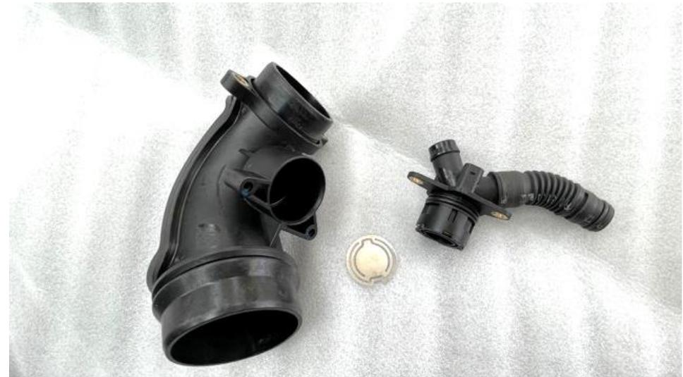
12. Remove the breather assembly from the inlet. There is also a metal shim inside the breather hole of the inlet.
