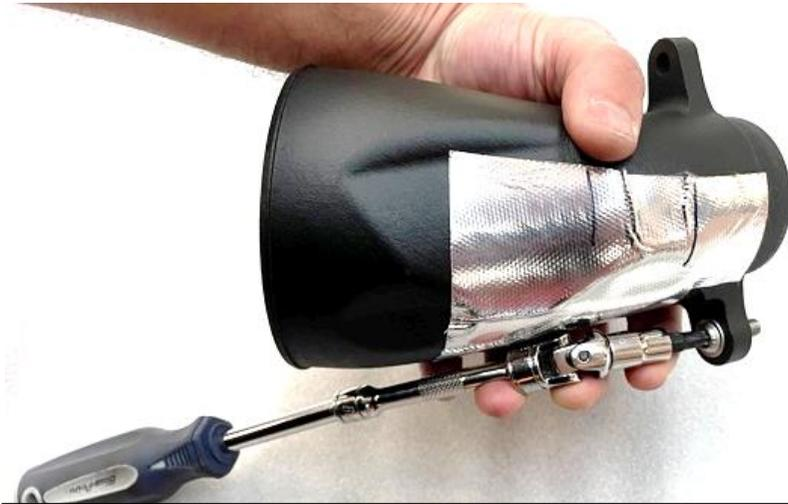
45. Accessing this screw with the inlet in place is tricky - we suggest to use a 1/4 " drive with a swivel socket located onto the screw as you lower it into place.
