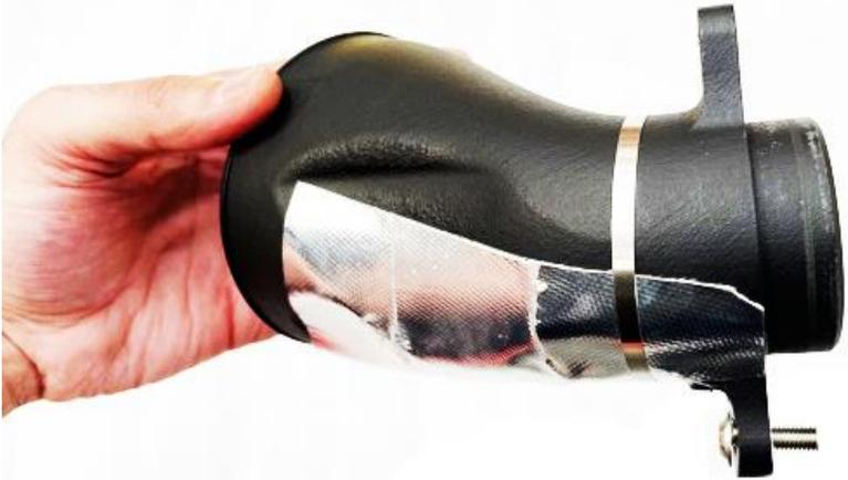
44. Take the LHS turbo inlet and push 1 x M6 Torx screw (provided) into the lower hole shown. There is also an O-ring inside the hole, make sure it stays inside.
