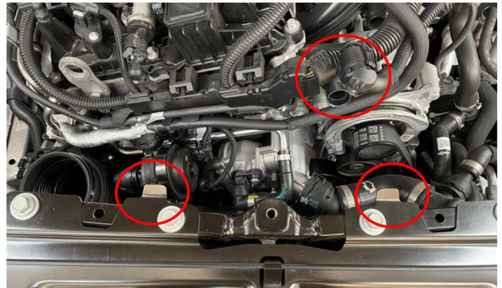
30. The back of the carbon duct secures into the OEM rubber grommet shown. Push the mount into the grommet.
