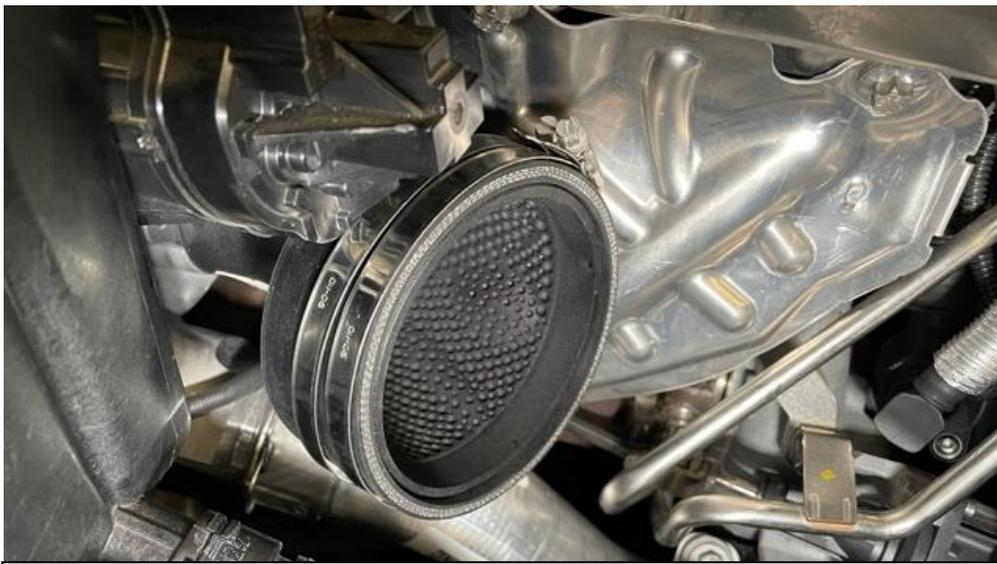
54. Take the remaining silicon hose and 2 x 90-110 clamps. Push the silicon all the way over the inlet - you need space to drop the filter housing into place.
