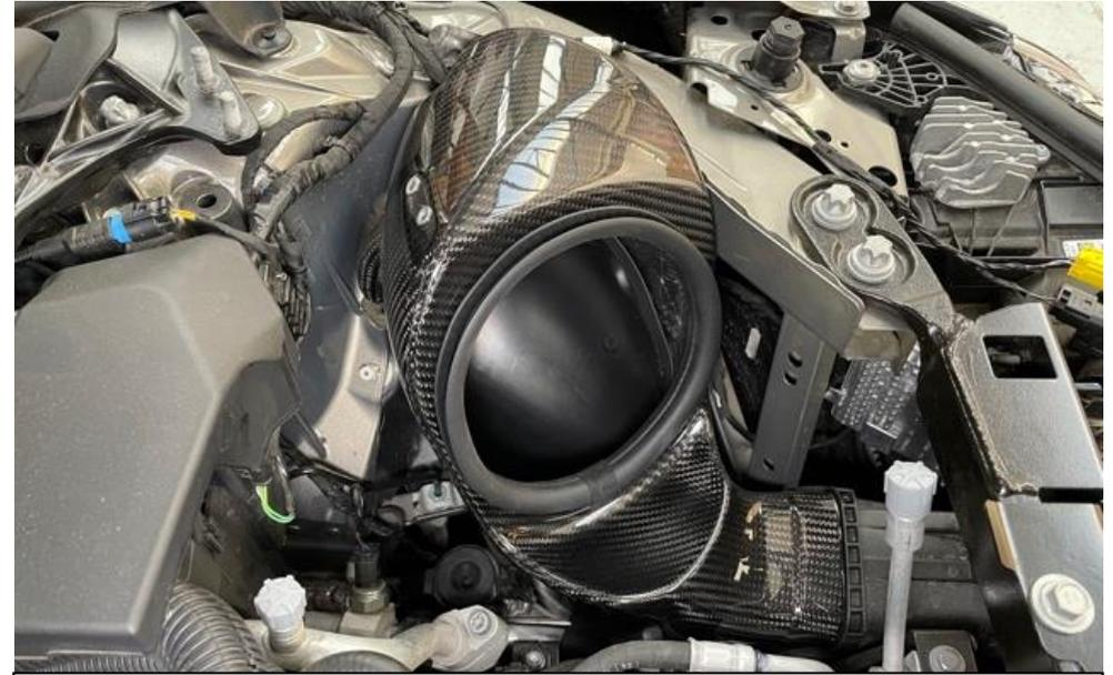
28. Identify the RHS carbon duct as shown.
