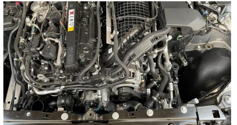
8. You can now remove the entire tube/airbox assembly from the car. The airbox pulls out.
