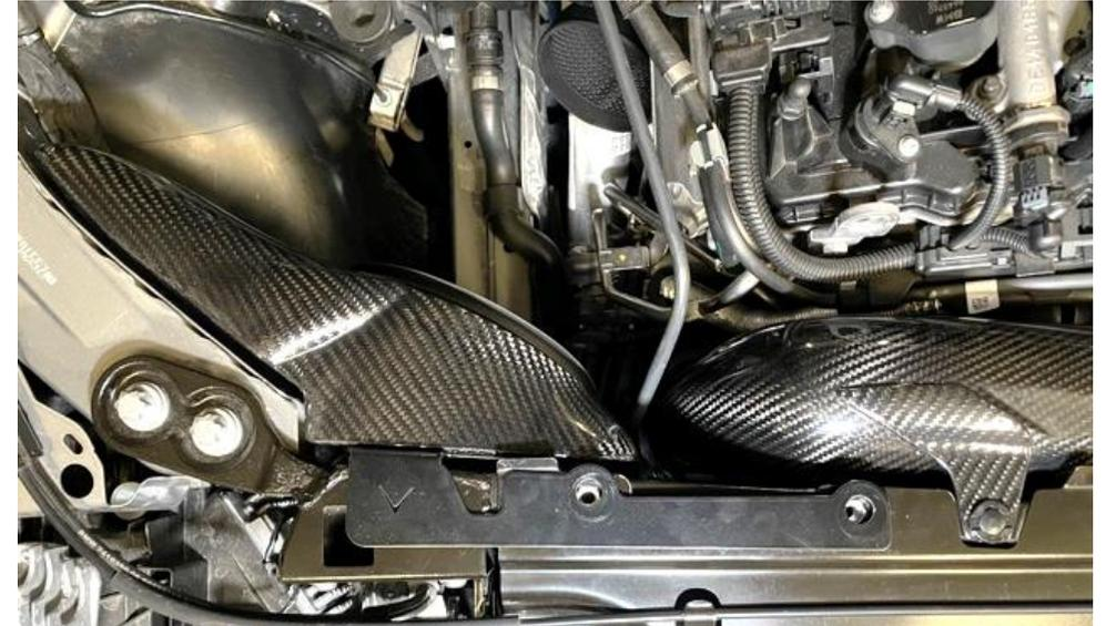
51. Position the duct so the bracket lines up with the 2 holes.
