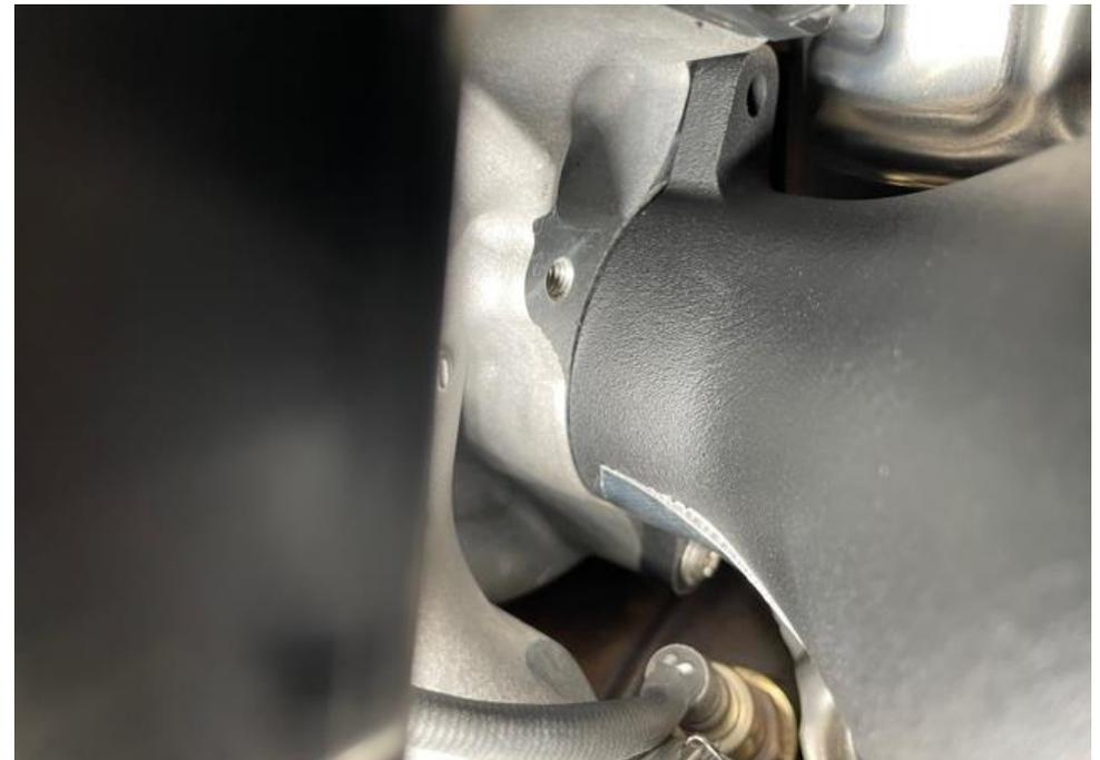
47. Continue to turn the screw while pushing the inlet further into the turbo until it sits completely in place and the screw is tight.
