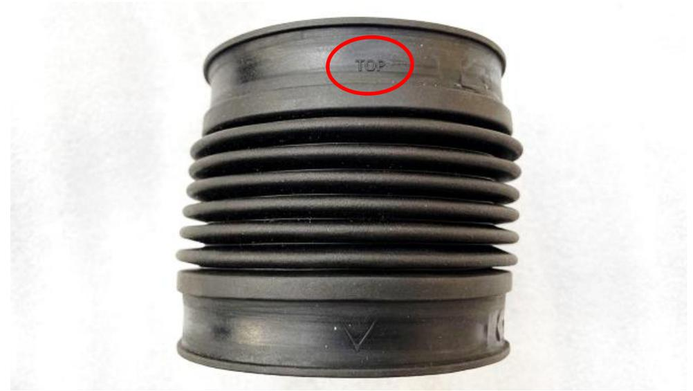
25. Take the new flexible rubber hose and identify the TOP as printed on the hose shown.
