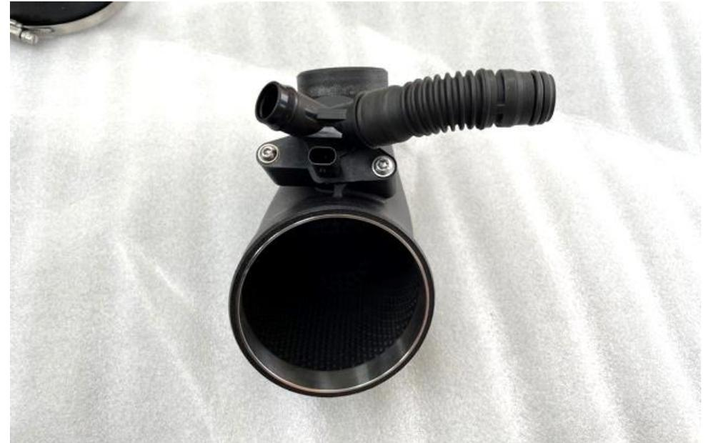
14. Secure the breather assembly onto the inlet using the OEM screws. **If the O-ring on the breather is too thick – please replace it with the one supplied in the kit.**
