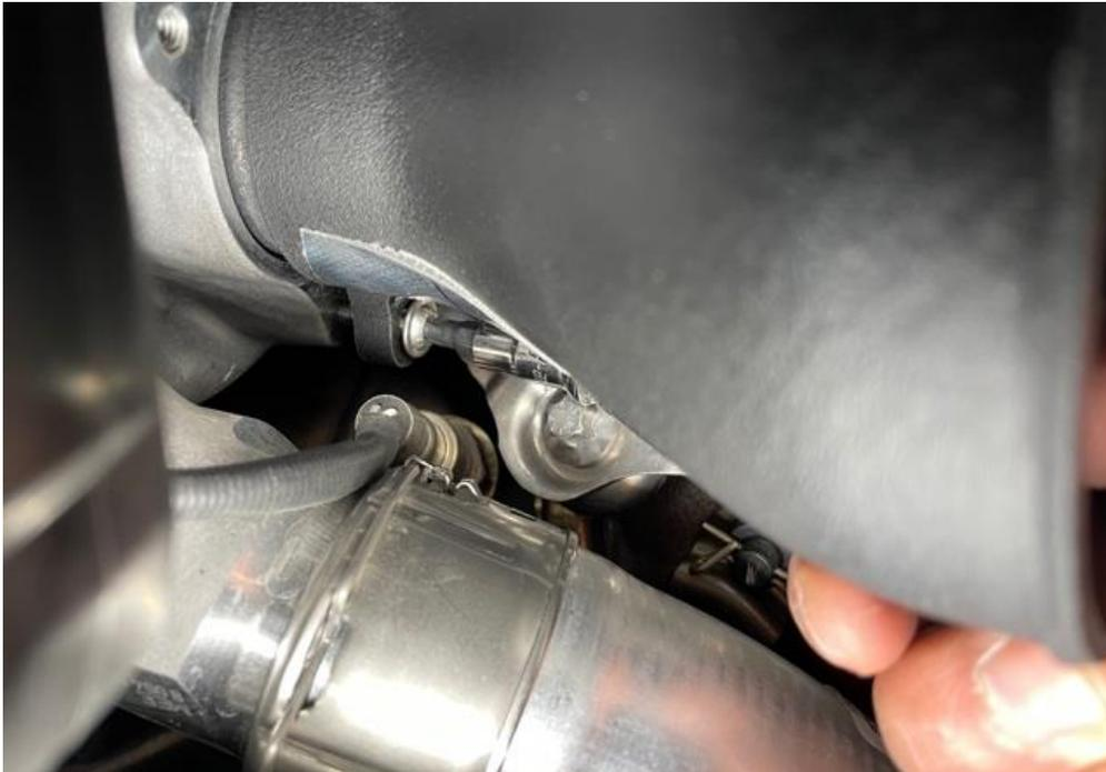
46. Locate the inlet into the turbo and carefully turn the screw as the inlet is gradually pushed into place.
