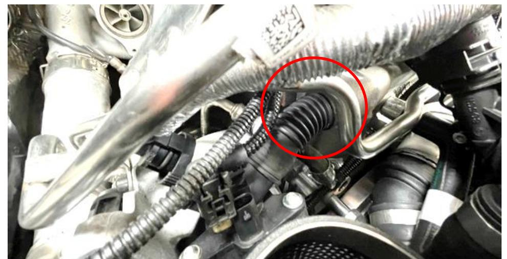
16. Push the breather back into place and secure with the clip. Push the inlet into the turbo fully.
