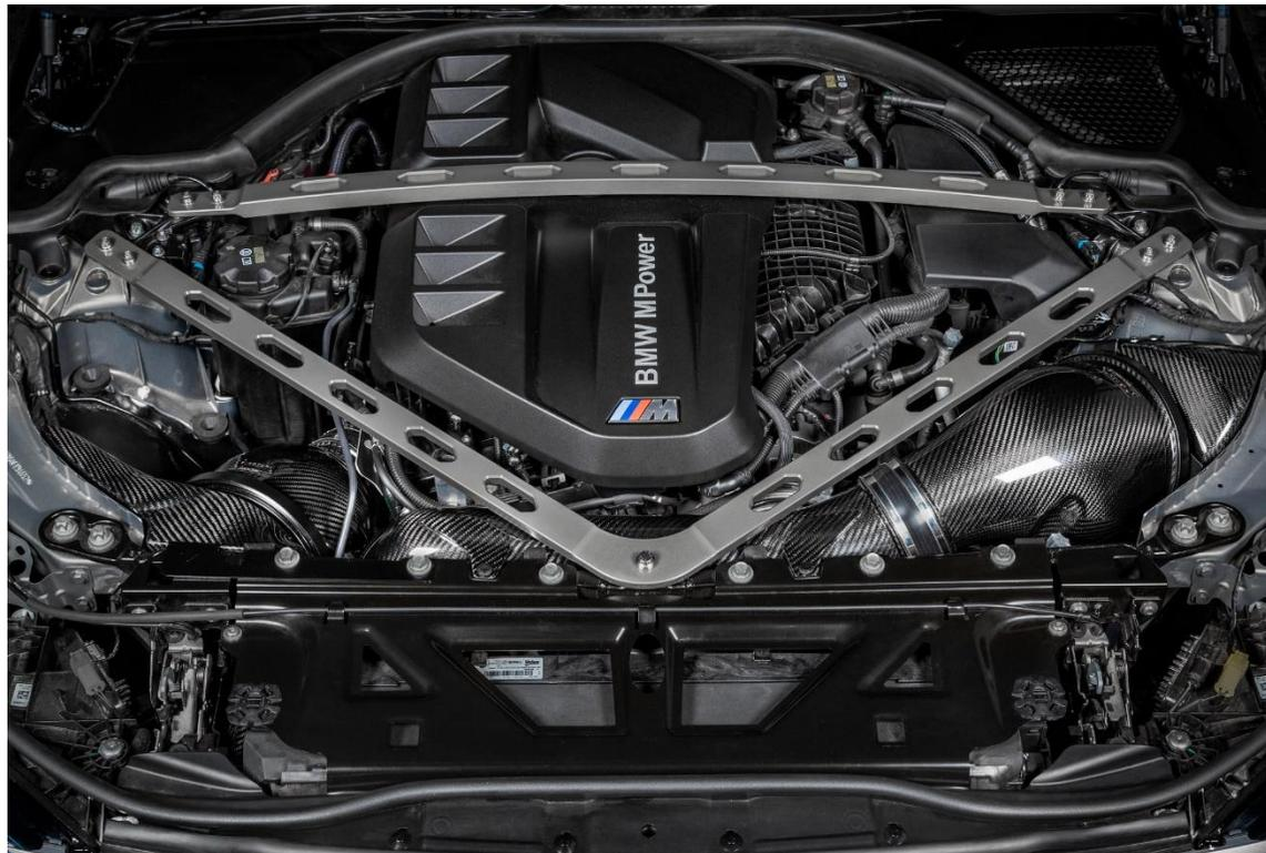
61. Assemble the engine cover and the strut braces back into position and tighten all bolts on the brace.
