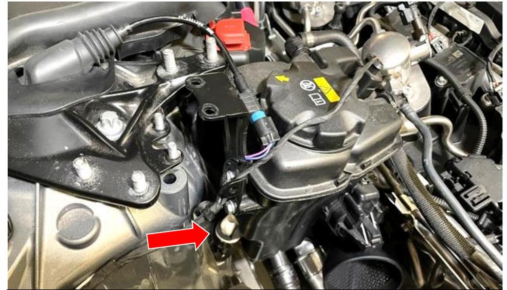
53. Lift the tank upwards and out of the white rubber mount as shown. Carefully rest it in place while the LHS housing is prepared.
