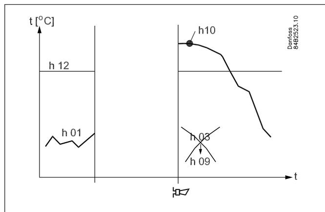
Exceeding in connection with power failure when the controller has lost its clock function and hence also its time performance.
