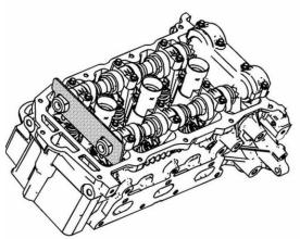
3. Install the en48383-3 to the rear of the right cam shaft
