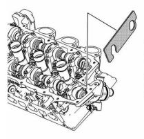
1. Install the en48383-1 to the left of the camshaft, make sure that the en48383-1 is completely on the camshaft
