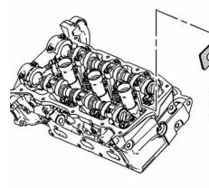
2. Remove the en48383-1 from the rear of the left camshaft, install the en48383-2 to the rear of the left side of cam wheel
