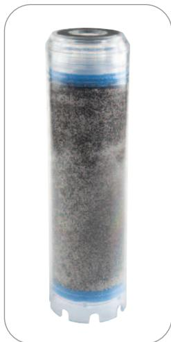
Plastic container filled with Pyrolusite for the reduction of dissolved iron and manganese (QA PRL) by oxidation and precipitation. Pyrolusite is not affected by the presence of chlorine in the water and is mixed with quartzite grit for better functioning.
