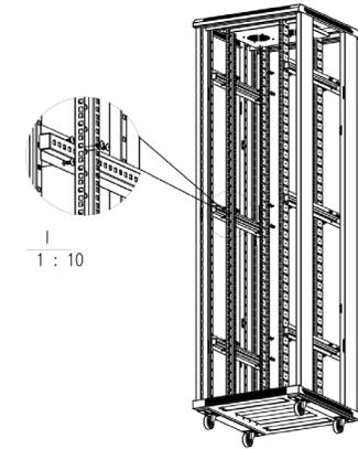
**I Step, Use M6\*12 Screw to fix the connect bar to the frame. And then use M6\*12 Screw to fixe the mounting elements to the connect bars.**
