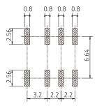
PC board mounting pad layout (TOP VIEW)
