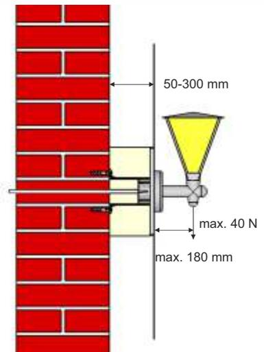
There is necessary to cut the carrier including inserted insulation before installation depending on layer thickness insulation.
