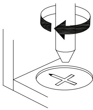
**EN** Turn cam lock clockwise to tighten.
