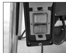
7. Switch-on (green)/ switch-off (red) – invisible on the first illustration
