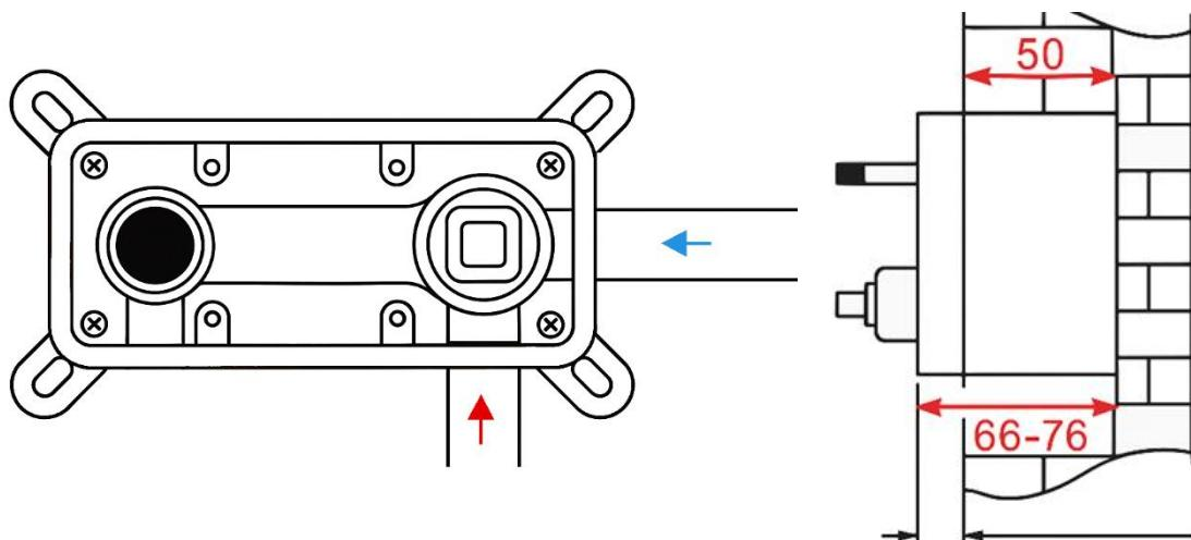
The total thickness of the finishing layer (e.g. tiles) should be between **66–76 mm** from the base of the mounting box.
