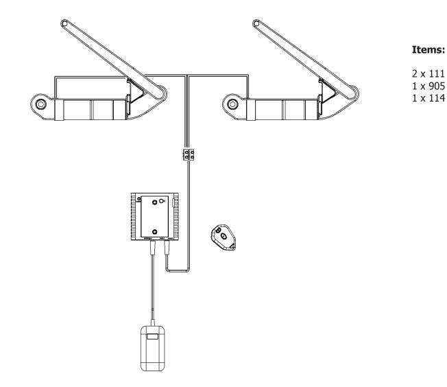
2 windows with 1 opener in each, auto-close remote controlled and with multiple channel remote.
