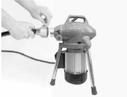
(5) Pull out a section (or less than 5 meters) of spring from the spring basket, take out the key used to remove the spring from the tool bag, insert it into the hole of the spring joint, and forcefully push it along the connection slot of the joint to remove the spring. (As shown in the figure)
