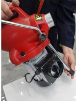
2. Fixed the 100 clutch handle, open the package and remove the machine, remove the dust bag, open the dredge head package, take out the hexagonal wrench, and tighten the screw to fix the clutch handle with the hexagonal handle.(as shown in the figure)
