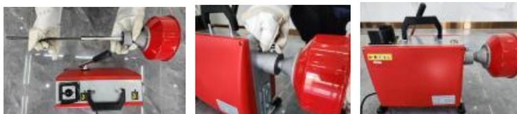
3. Place the machine 1-2 feet away from the inlet of the pipeline, as excessive distance can cause steel cables to entangle.
