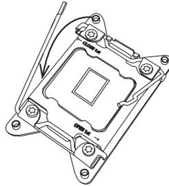
3. With the lever labelled 'Close 1st' fully retracted, gently push down on the lever labelled 'Open 1st' to open the load plate. Lift the load plate to open it completely.
