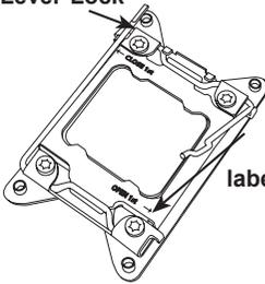
Push down and lock the lever labelled 'Open 1st'.
