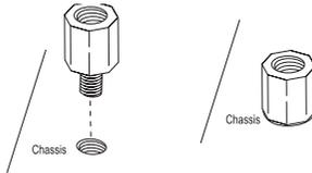
5. Install the motherboard into the chassis carefully to avoid damaging motherboard components.
