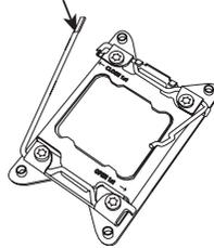
8. Close the load plate with the CPU inside the socket. Lock the lever labelled 'Close 1st' first, then lock the lever labelled 'Open 1st' second. Using your thumb gently push the load levers down to the lever locks.
