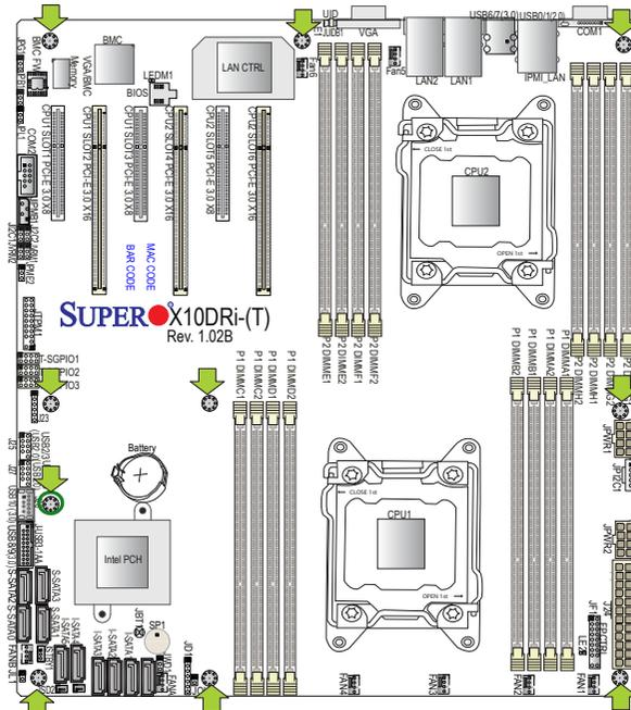
**Caution:** 1) To avoid damaging the motherboard and its components, please do not use a force greater than 8 lb/inch on each mounting screw during motherboard installation. 2) Some components are very close to the mounting holes. Please take precautionary measures to prevent damage to these components when installing the motherboard to the chassis.
