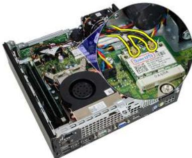
6. Push the securing levers away from the WLAN card.
