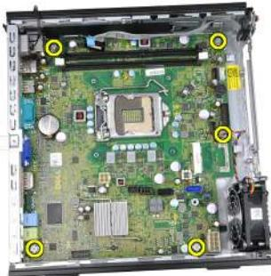
14. Remove the 7-mm hex screw from the system board.
