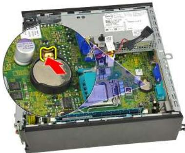
7. Lift the coin-cell battery out of the computer and properly dispose of the battery.
