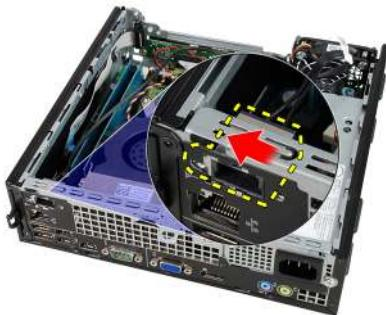
8. Remove the internal antenna.
