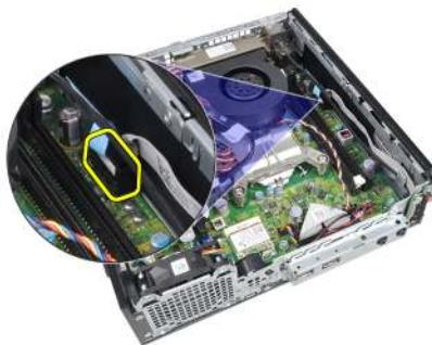
7. Unthread the control panel-speaker cable from the chassis clip.
