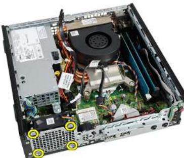
8. Lift and remove the system fan out of the chassis.
