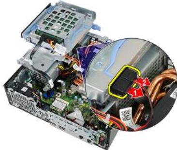
6. Remove the data cable and power cable from the back of the hard drive.
