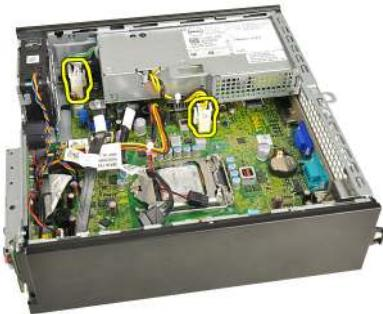
8. Remove the screw that secures the power supply to the chassis.
