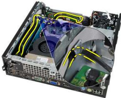
7. Release the internal antenna port.
