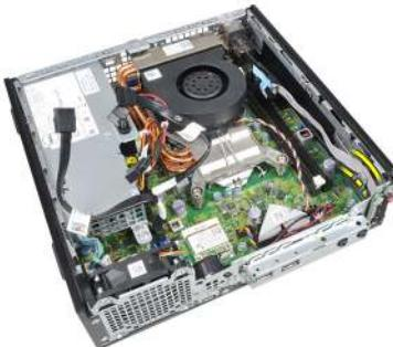
8. Remove the screw that secures the control panel board.
