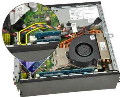
6. Press the release lever down and move it outward to release the fan retention hook that secures it.
