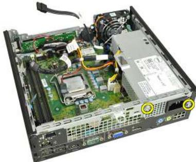
10. Slide the power supply inward and remove the power supply.
