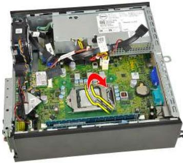
8. Lift the processor to remove it from the socket and place it into an antistatic packaging.
