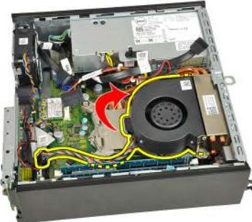
8. Loosen the captive screws to secure the heat sink/fan assembly to the system board.
