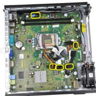
12. Unthread and move the internal antenna from the chassis.
