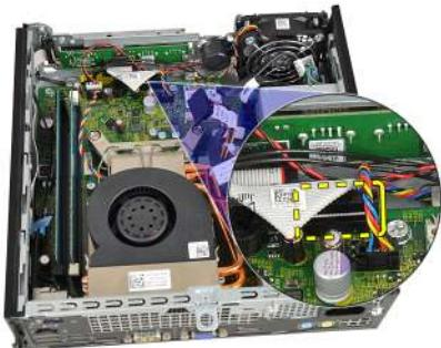
6. Remove the screws that secure the Input/Output bracket.
