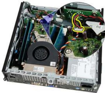
6. Pull out the speaker cable from beneath the system fan cable and wireless local Area network (WLAN) antennae (if installed).
