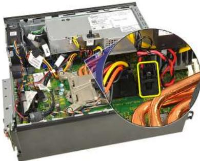
6. Slide the intrusion switch over and remove it off the bracket.
