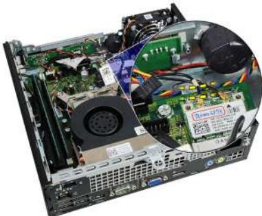
7. Remove the screws that secure the fan to the chassis.
