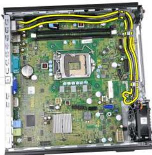
13. Remove the screws that secure the system board to the chassis.
