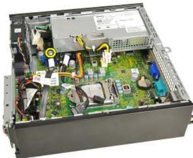
9. Remove the screws that secure the power supply to the chassis.
