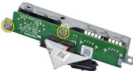
9. Remove the Input/Output bracket.
