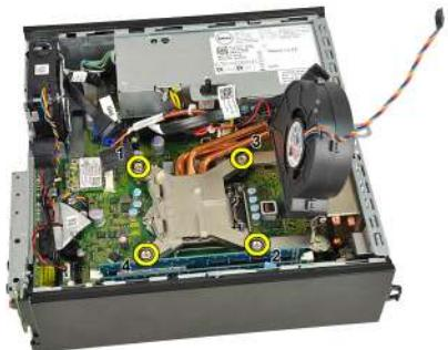
9. Lift the heat sink/fan assembly upward, and remove it from the computer. Lay the assembly with the fan facing downward, and with the thermal grease facing upward.
