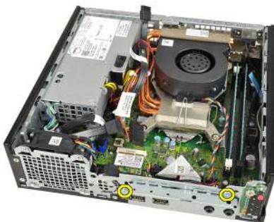
7. Remove the Input/Output bracket from the chassis.
