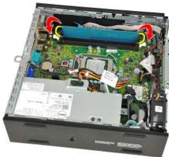
6. Lift the memory module out of the connector on the system board and remove it.
