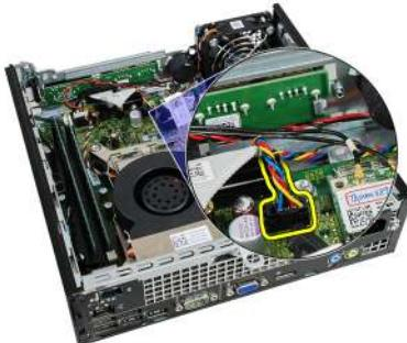
6. Disengage the system-fan cable from the chassis.
