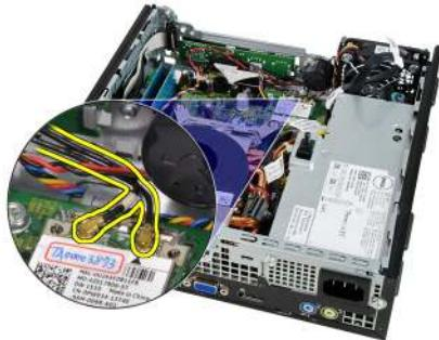
6. Unthread the internal antenna.
