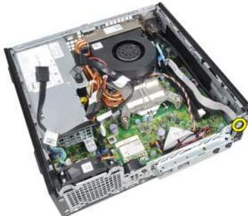
9. Remove the control panel board.
