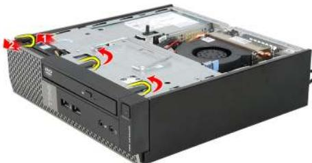
4. Rotate the bezel away from the computer, to release the hooks on the opposite edge of the bezel from the chassis.
