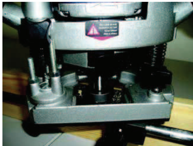
Fig.8. Milling holes 23x60x30 using three passes.
