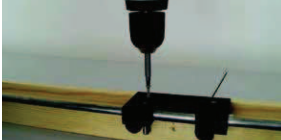
Fig.6. Screwing down frame with screws.
