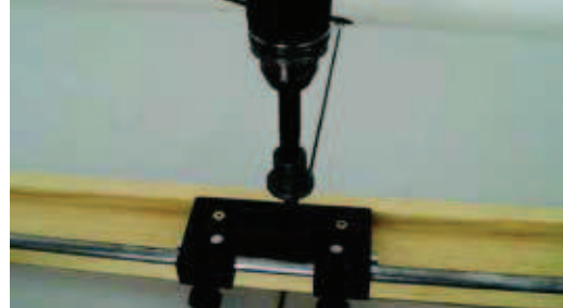
Fig.7. Drilling lead hole with d.12,5 drill.
