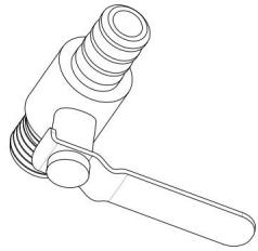
A line drawing of a ball valve, showing a handle attached to a U-shaped valve body with a spherical seat inside.                                       |
